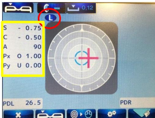
In this case the Lens Meter should read 1D Base Out and 0D Base Up/Down
