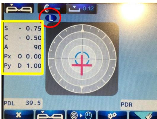
In this case the Lens Meter should read 1D Base Up and 0D Base In/Out
